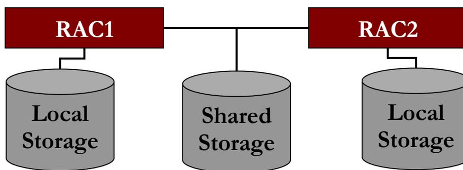
The diagram above shows a simple RAC cluster architecture. A minimal cluster consists of multiple servers, a private network, a public network, and shared storage. Most DBAs are familiar with the single-instance configuration in which storage is not shared between nodes and all access to the database comes from the single instance.
