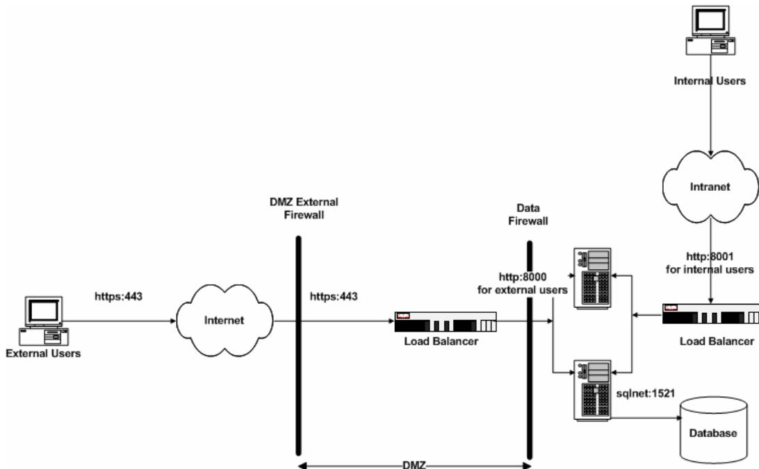
**Figure 5 – Hardware Load Balancers without an External Web Server**
