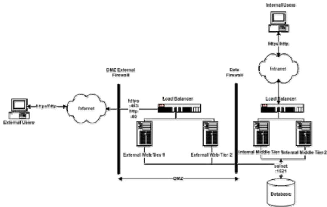
**Figure 4 – Hardware Load Balancers with an External Web Server**
