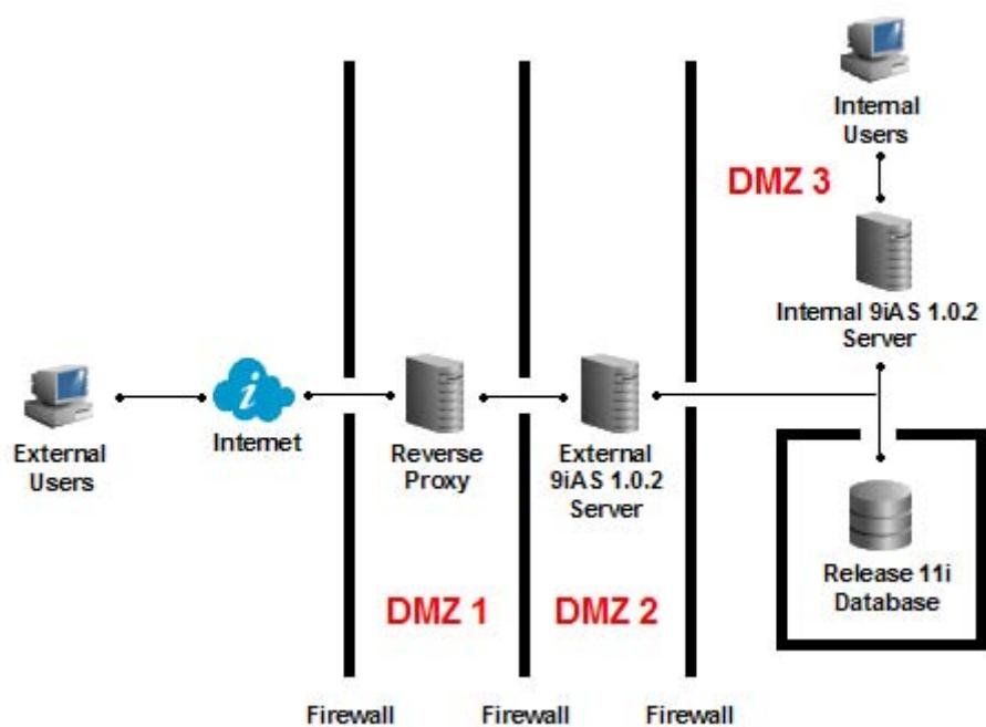
Figure 1 – Reverse Proxy with an External Web Server
